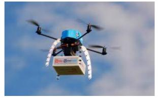
Munoz made the drone's autopilot system by taking the motion sensors from a games console remote control. To attach the microchips to circuit boards he heated them up in a domestic oven.
